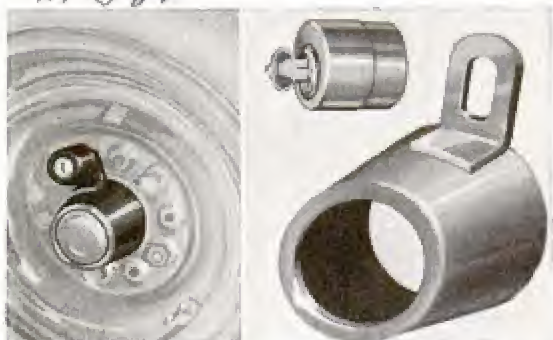
Note how lock covers hub so wheel can't be removed
